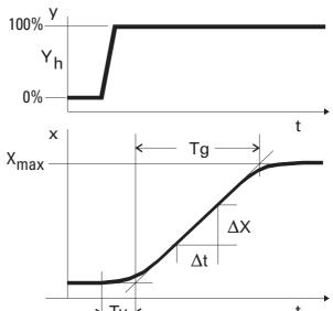
$$\begin{array}{rcl} y & =& \text{correcting variable} \\ Y_h & = & \text{control range} \\ Tu & = & \text{delay time (s)} \\ Tg & = & \text{recovery time (s)} \\ X_{max} & = & \text{maximum process value} \end{array}$$
